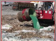
350 degree rotation allows for barrel to be easily unloaded.
