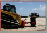
Tool head rotates 175 degrees to the left and right.
