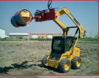
The Barrel Handler attaches to all machine
