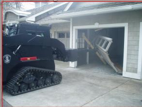
Tear down doors and walls and stop vehicles in their tracks with the Rotating Scorpion Tool.
